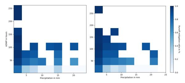
Fig. 4: Ratio between mitigated runoff in relation to ADWP (the period between two independent rainfall events) in hours, and precipitation per rainfall event in mm on green roofs in the year 2020 (left) and in the year 2050 (right).
