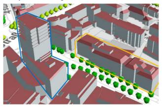
Fig. 3: Buildings from case study area of different geometry with similar volume to ground area ratio. Source: LHS Stuttgart, Stadtmessungsamt
