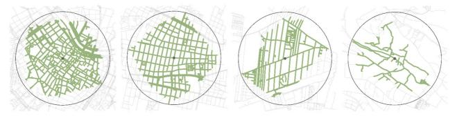
Fig 3: Permeability of different urban structures in Vienna, illustrated by the comparison of a 800 meters radius and the actual network covered with a travel distance of 800 meters in each structure respectively © Tobisch
