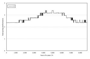
Fig. 10: Performance of chosen river water heat pump.
