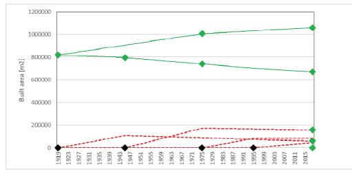
Fig. 6: Scheme for estimating the built area per construction period. The green colored datapoints orginate from the GIS analysis and act as input data for the model. The temporal developments of the built area per construction period (red dotted lines) are unknown.
