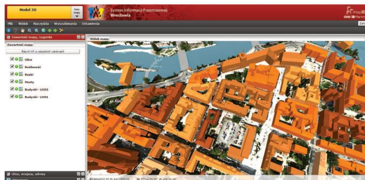
Fig. 9 3D model of the City of Wrocław, a 3D module of the city geoportal.
