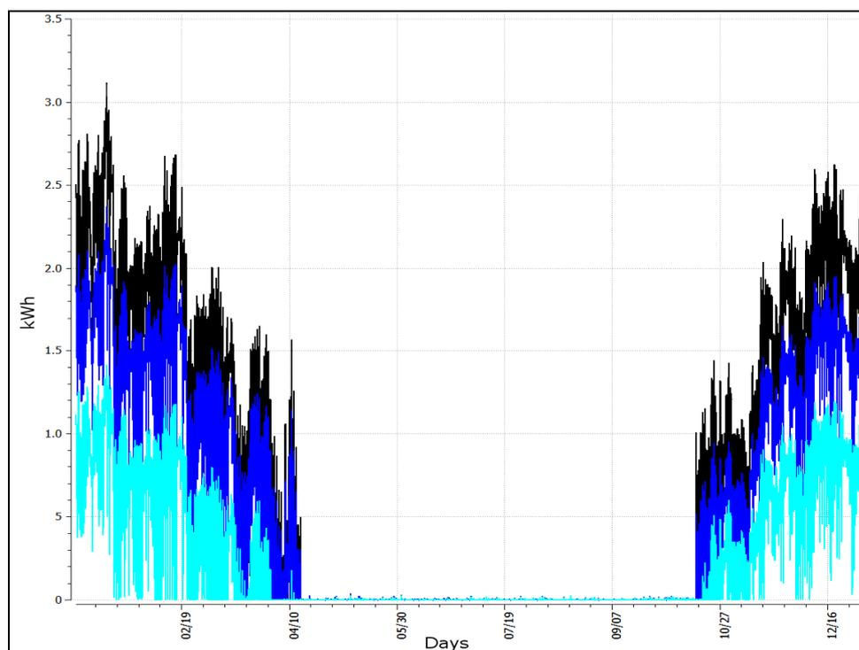
Fig 6: Plot of the hourly energy demand values for one zone. As elsewhere in this paper, the different colours correspond to the three different scenarios: black “as built”, blue “current state”, azure “refurbished state”.
