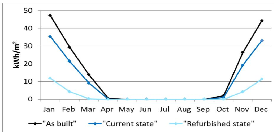
Fig. 4: Plot of the monthly net energy demand values for space heating for the building depicted in Figure 3 (left) are presented. As elsewhere in this paper, three different scenarios were computed.
