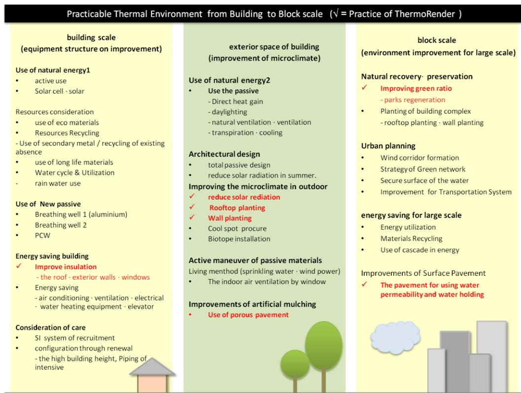
Fig. 3: Thermal environment measures of according to the scale.
