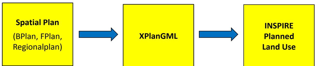
Figure 4: Automatic transformation of spatial plans into the INSPIRE PLU format
