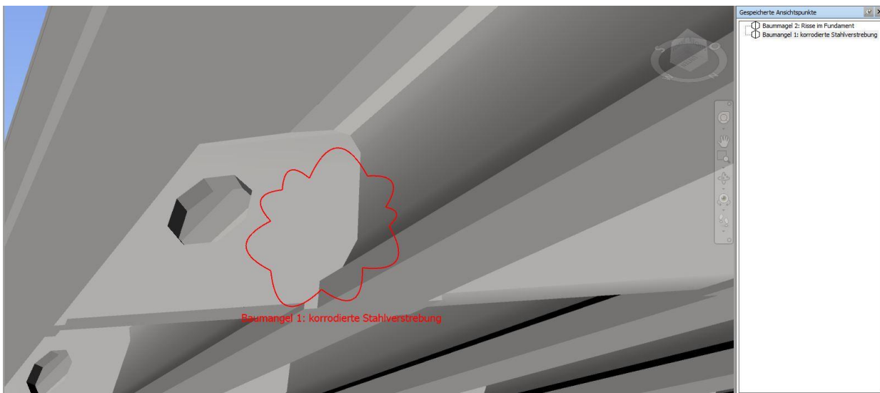
Fig. 2: Screenshot from Autodesk Navisworks for visualizing construction damages (Own source)
