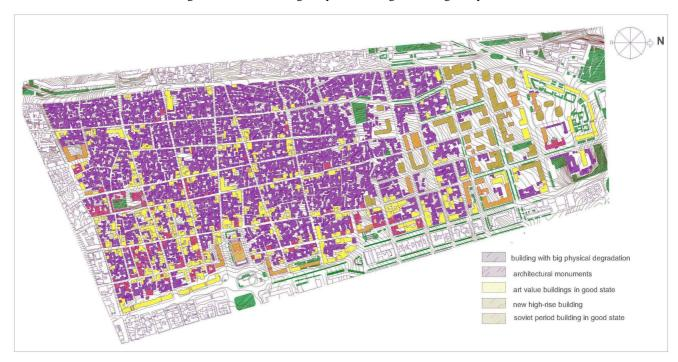
Fig. 7: Scheme of building analysis according to art value
