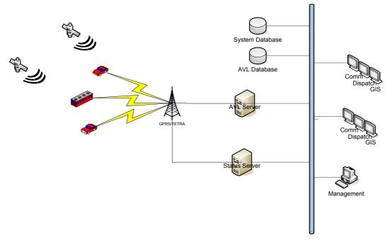
Figure 5 Simplified ALV Schema
