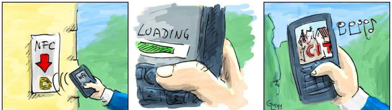
Fig. 3: Functional principle of the NFC system (contacting – decoding – playing) – source: Own figure
