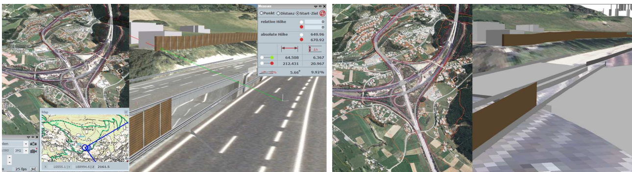
Fig. 1: Comparison of GEARViewer and ArcScene at 2 levels of detail. Left: GEARViewer showing 5cm orthoimage overview and close up (with line of sight GUI); Right: ArcScene with same dataset and viewpoints at maximum capacity
