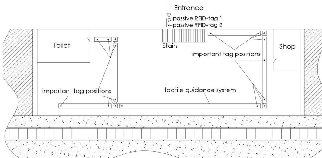
Fig. 1: Routing by tactile guidance system and RFID-tags
