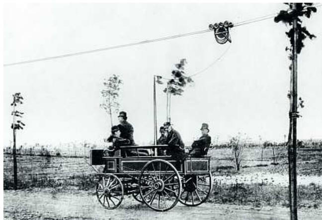
Fig. 1: Elektromote of Werner Siemens
