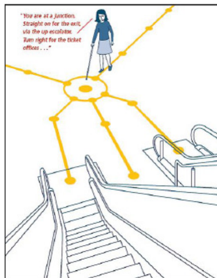
Fig. 2: Application of RFID-tags as guidance system for the blind and visually impaired (Gill, 2007)
