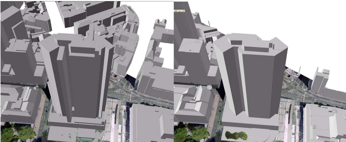
Fig. 9 Rectangle Segmentation (left) and Cell Decomposition (right)
