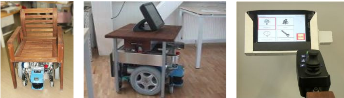
Fig. 2: The MOVEMENT modular prototype consists of a semi-autonomous robotic platform able to dock to various application modules like chairs, tables, ICT terminals and thus can provide mobility of persons, objects and information (left: robotic mobility platform moving a chair, middle: platform fetching a table with ICT terminal, right: touch screen and joystick for assisted driving mode).
