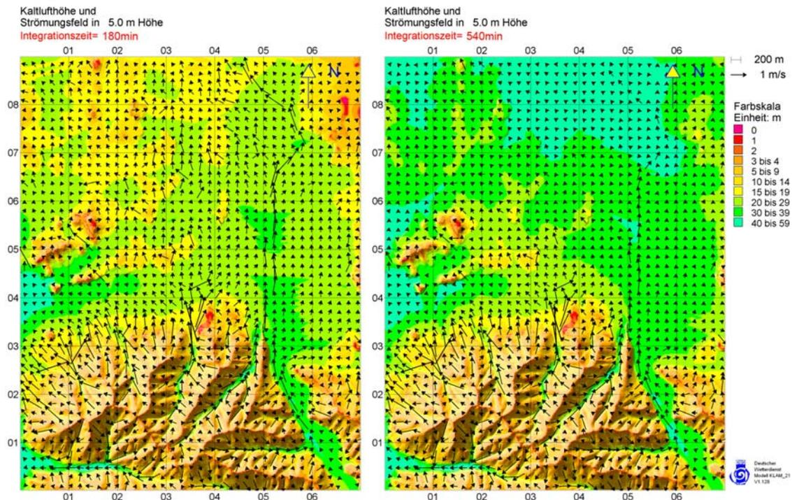
Figure 9. Wind Corridor Simulation of Target Area (3 hours passed, 9 hours passed)
