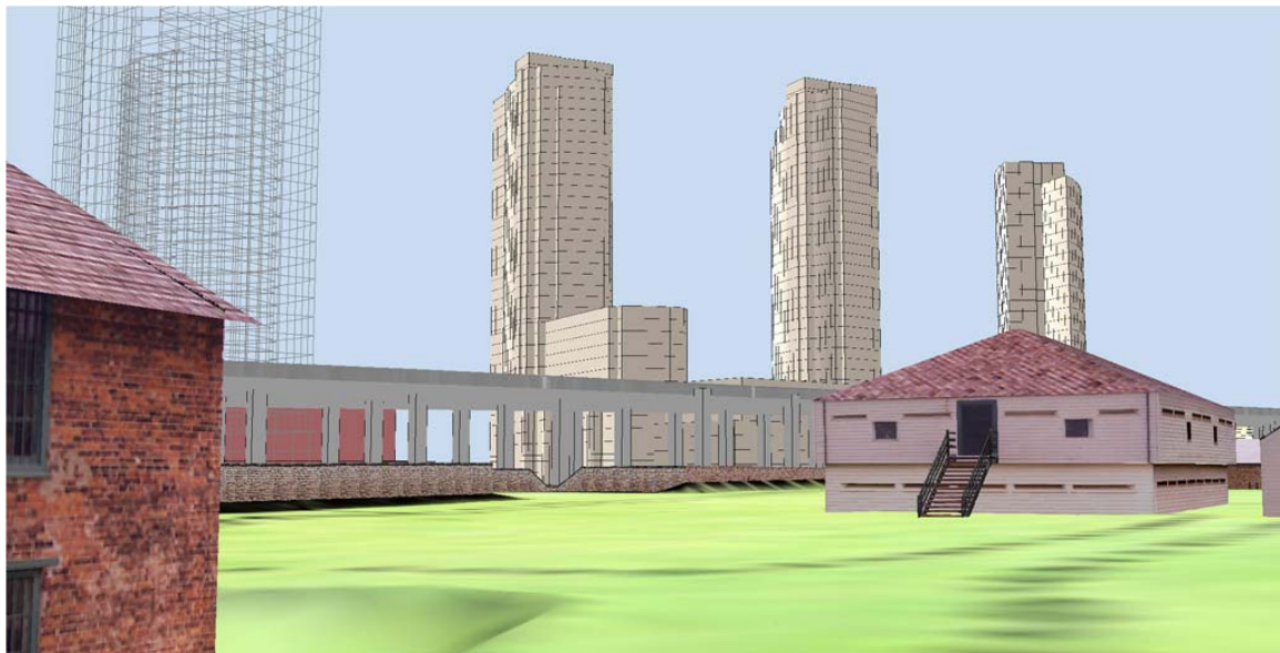
Figure 4: Comparative overlay of the developers favored tower typology (wire frame) and the equal density medium height typology developed by local volunteer urban design professionals (solid)
