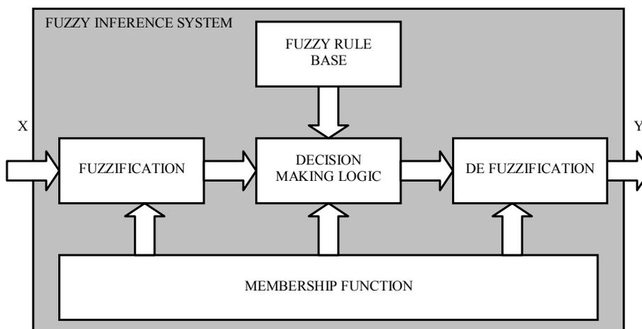
Figure5: Block structure of Fuzzy system
