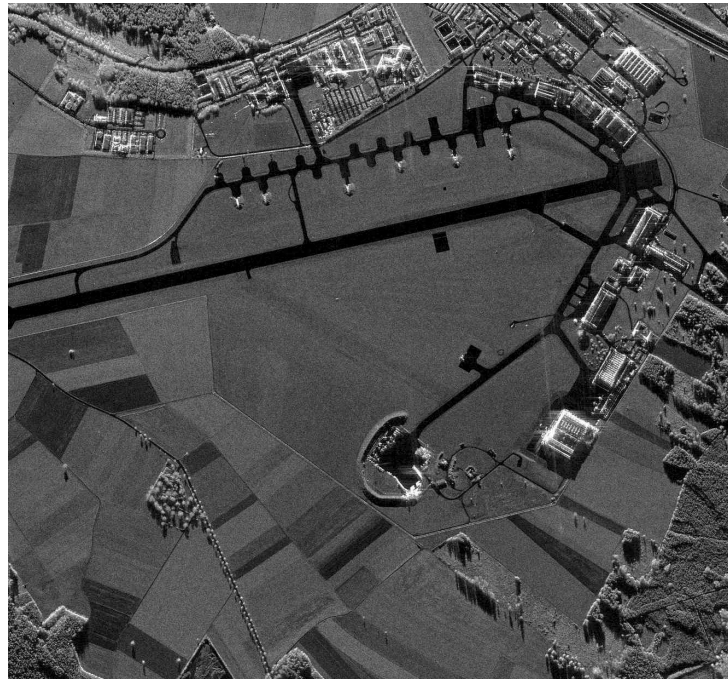
Fig. 2: The airport of Oberpfaffenhofen with DLR research centre on top – X-band data at 1 m resolution provided by the airborne Do-SAR
