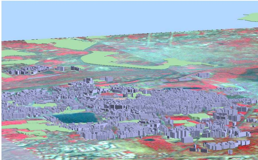
Figure 4. Extruded buildings using the height information from Cartosat-1 images (displayed on the Resourcesat image)
