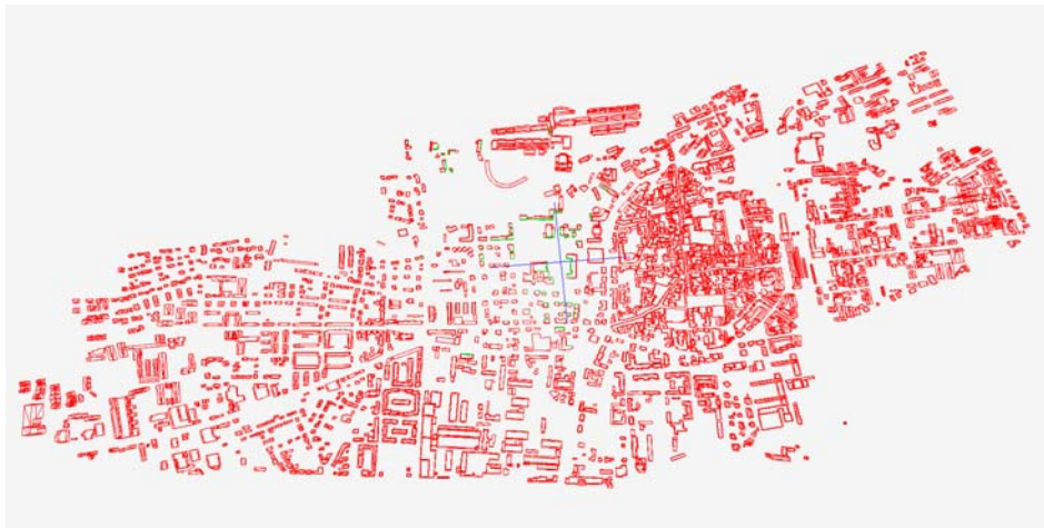
Figure 4: Map of a city with a marked location based service query point and the query result of all triangles found to be visible drawn in green.
